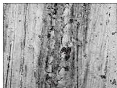
Photo 2 Peeling failure after refrigerant environment testing
