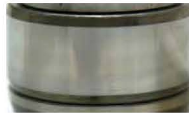
Photo 2 Inner ring raceway of a newly developed bearing after skidding test
